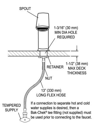
Solenoid carrier includes strainer for easy above deck service. Thermostatic mixer ordered separately to comply with ASSE 1070 requirements. The product shall be tested and certified to industry standards: ASME A112.18.1M, CSA B125.1, California Health and Safety Code 116875
