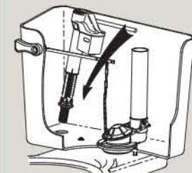
**c) Press down until corner of silver cover and top of flush valve (FV) line up.**
