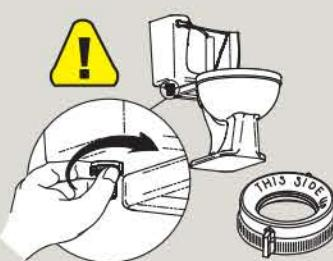
**b)** **Confirm critical level (C/L) is 1" above flush valve (FV).** Code requirement.
