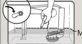
**c) Remove old flapper. Install new flapper with minimal chain slack (S).**
