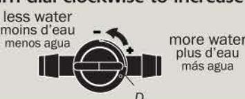
**c)** Repeat 8b until bowl water level reaches pencil mark at the same time tank finishes filling.
