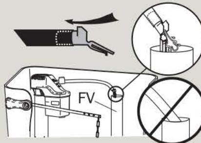
**7**) Connect water supply. Do not use sealant or tape. **Hand-tighten only.**
