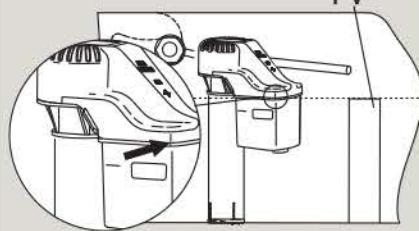
**6**) Install mounting nut. **Hand tighten only,** beveled side up.
