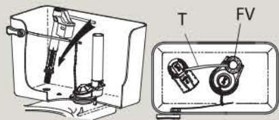
**c)** Verify corner of silver cover & flush valve (FV) line up.
