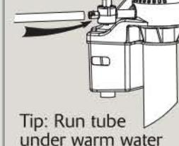
Tip: Run tube under warm water for easier install.
