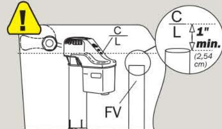
**c)** Attach tube to flush valve (FV) with metal clip so water flows into flush valve. Trim tube if kink occurs.
