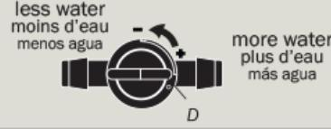
d) Repeat step C until bowl water level reaches pencil mark at the same time tank finishes filling.
