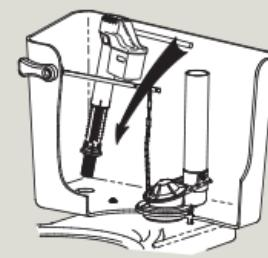
**3 a)** Press down until corner of blue cover and top of flush valve (FV) line up.
