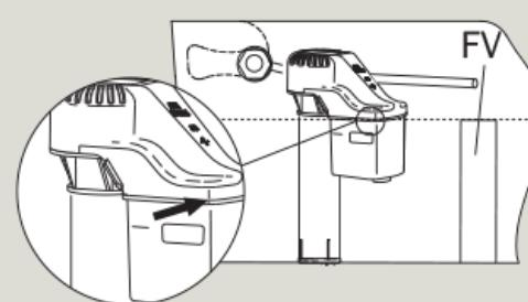
**c)** Install mounting nut. Hand tighten only, beveled side up.
