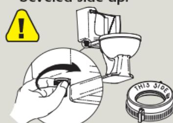
**5 a)** Confirm critical level (C/L) is 1" above flush valve (FV). Code requirement.
