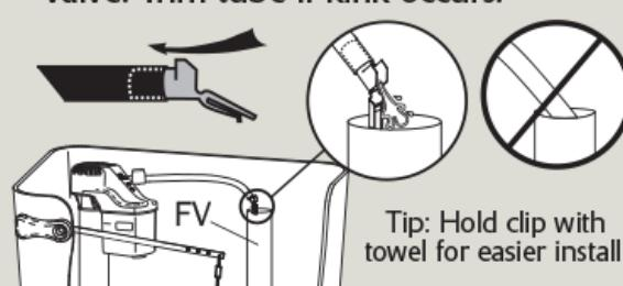
**c)** Caution: Push tube as shown to ensure port is locked in place.
