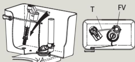
**b)** Verify corner of blue cover and top of flush valve (FV) line up.
