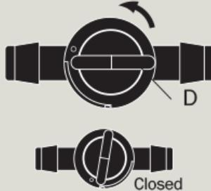
b) Locate adjuster key setting from Fit Chart below and place on ledge (L) as shown. Adjust amount of refill water by turning adjuster dial (D) clockwise until it contacts adjuster key.
