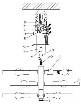
Important Note: To avoid snapping the fixture's wires, do not fully twist the rings more than 2 times in the same direction. Instead twist the ring in the opposite direction to achieve the look you desire.
