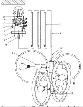
Important Note: To avoid snapping the fixture's wires, do not fully twist rings (H) more than 2 times in the same direction. Instead twist the rings in the opposite direction to achieve the look you desire.
