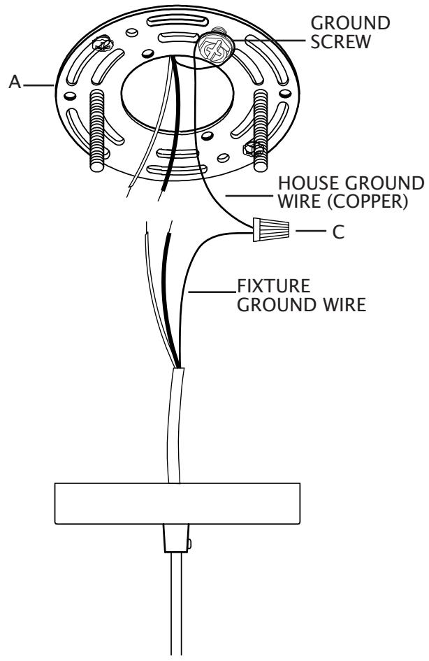
10. Twist end of house lead wire (black) and end of fixture lead wire together. Twist wire nut (C) onto ends of wires. Completely tighten wire nut (C). Twist end of house neutral wire (white) and end of fixture neutral wire together. Twist wire nut (C) onto ends of wires. Completely tighten wire nut (C). Reference chart to the right for correct wire connections.
