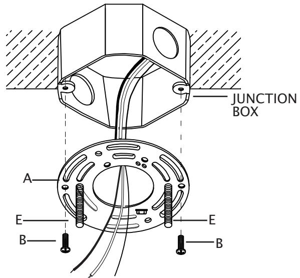
6. The length of the cord must be adjusted before fixture is installed. Hold canopy (D) against ceiling to determine desired hanging height of fixture.
