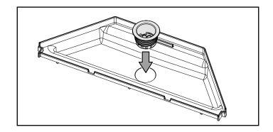
4. Install the O-ring over the strainer threads.
