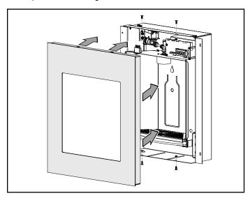
Attach the front cover with the top two mounting screws to prevent it from falling away from the water dispenser while the filter unit is being installed.
