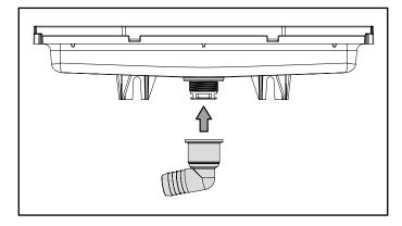
NOTICE For the following steps, it is recommended to use a heat gun when manipulating the flexible drain hose. It is beneficial to conservatively soften the material before trying to make connections.
