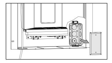
regulations and standards when connecting any electrical device. A minimum 15 AMP GFCI Circuit Breaker is required for safe installation.
