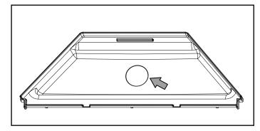
Trial fit the strainer. If the strainer does not fit, carefully open the size of the hole. If it fits well, place a small amount of plumbers putty around the lip of the strainer flange and insert it into the hole.
