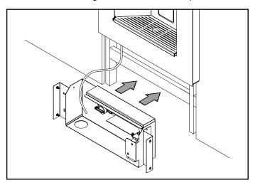
3. Using four #8 flathead screws, start the screws to hold the unit in place.
