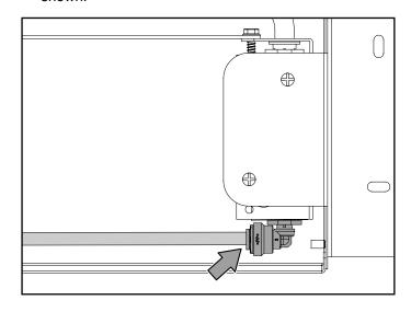
9. Connect an installer supplied 3/8" water supply tube to the quarter-turn shutoff valve, as shown. The type of tubing, copper or plastic, should meet all local regulations and building codes.
