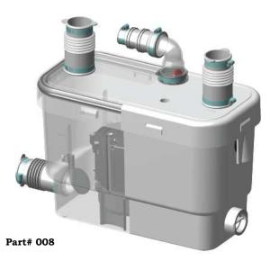
The Sanivite is a gray water pump that is ideally suitable for use in a basement apartment or anywhere in the house where additional fixtures are most wanted. It will pump waste water away from a variety of sources such as: a kitchen sink, laundry sink, washing machine (indirect connection), dishwasher, bar sink, etc.
